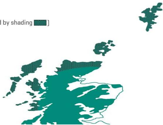
Due to the exceptionally high wind loads which are experienced on the Scottish Islands and exposed Coasts, specific recommendations are required for the use of fibre cement profiled sheets as detailed below. These recommendations should be considered as the minimum requirements for fixing sheets in the shaded area of the map, but where design wind loads exceed 2.5kN/m<sup>2</sup>,
