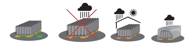
When the sheets are delivered, the packaging must be removed, the sheets must be left on the pallet and firmly stored on solid ground. Sheets cannot be stored in an open space, sheets should be placed under shelter, and if there is no possibility to do this, we recommend covering loosely with a weather resistant tarplin to protect it against the weather elements.
